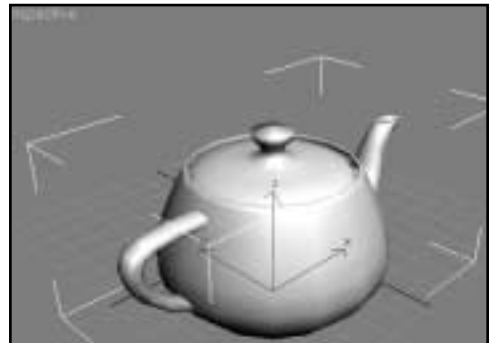
Figure 2.10 The quickest way to create a mesh object is to click and drag.
