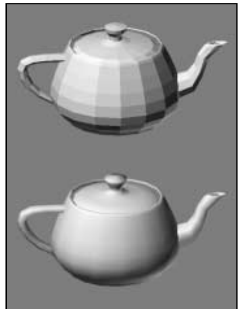
Figure 2.19 When a mesh object is smoothed, edge divisions disappear. Above: a teapot with unsmoothed faces. Below: a teapot with smoothed faces.
